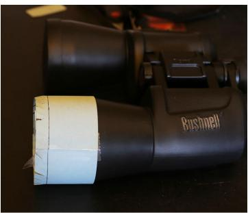
Place the paper tube on the piece and fold the cut tabs parallel to the lens.
