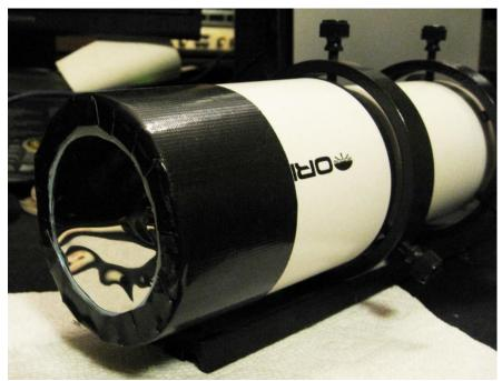
If the filter fits loosely, you can fold tape over the open end of the tube, to make it fit more snuggly. Always hold the filter up to the light to check for pinholes. If you see light don't use the filter.
