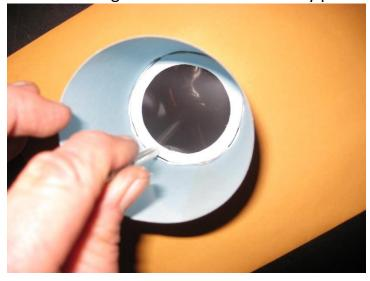
If you used tape, the following doesn't apply. If you are using a telescope, you can place the filter on the scope and place the filter down, using the weight of the scope to press on the filter to allow the glue to dry. It's best not use a camera lens this way, because any excess glue could stick to the lens cap. With the filter side down place something flat across the open end and put something relatively heavy on top. Big meteorites work well.
