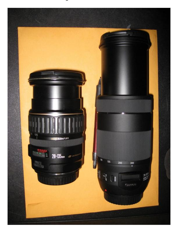
Extend the lens to maximum zoom, lay the lens across the width of cover stock, leaving about a half inch space at the front of the lens. The paper needs to cover the control ring so it rotates with the filter in place. Then draw a line across the height of paper at the back of the front control ring.
