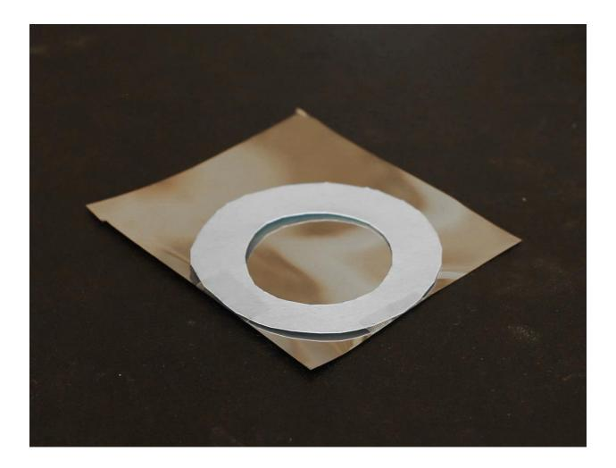
Next, apply the double-sided tape, all the way around, to one side of the rings. Place the solar material on a sheet of paper, or paper towel. Place the ring on to the filter material with taped side toward the filter material. Press the ring firmly to the filter material. Flip it over and repeat the process with the other taped ring.
