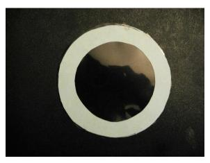
Next, make sure that you can place the filter inside the tube without it folding or bending. You may have to trim the outside to make it fit. Be careful not to touch the filter material. You could use the double-sided tape, but I prefer using a small amount of glue towards the outside of the ring, with the silver side up.
