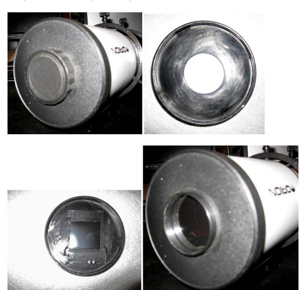
Cut a piece of solar film larger than the hole and tape it to the inside, with the silver side facing the Sun. That's all there is to it, make sure it's on the telescope, before you point the telescope at the Sun.
