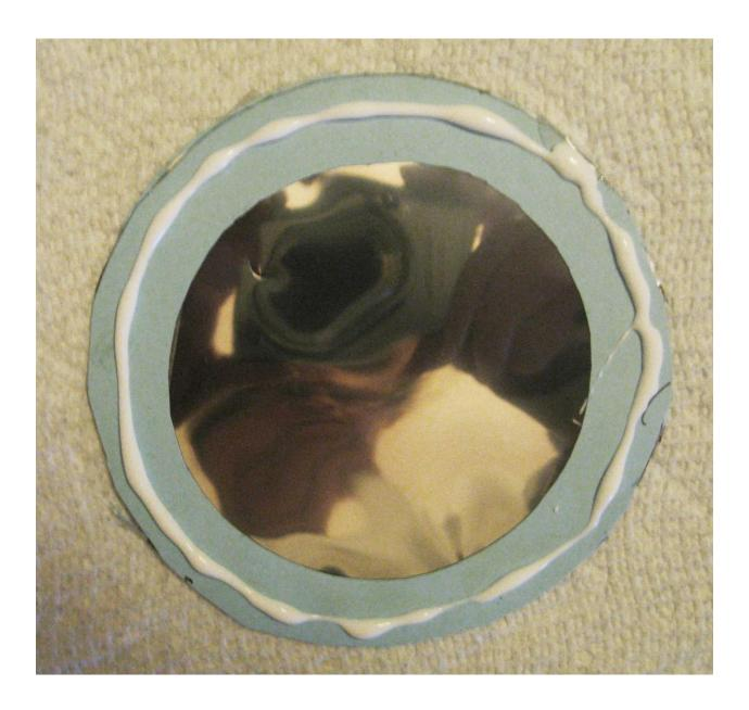
With the tape or glue side down, place the filter inside the tube, shiny side out, Use something with a blunt end to firmly press the filter in place.
